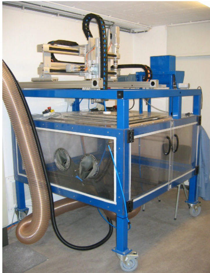
Fig. 2. The blasting cabinet for micro abrasive air jetting, with traversing system on top.
