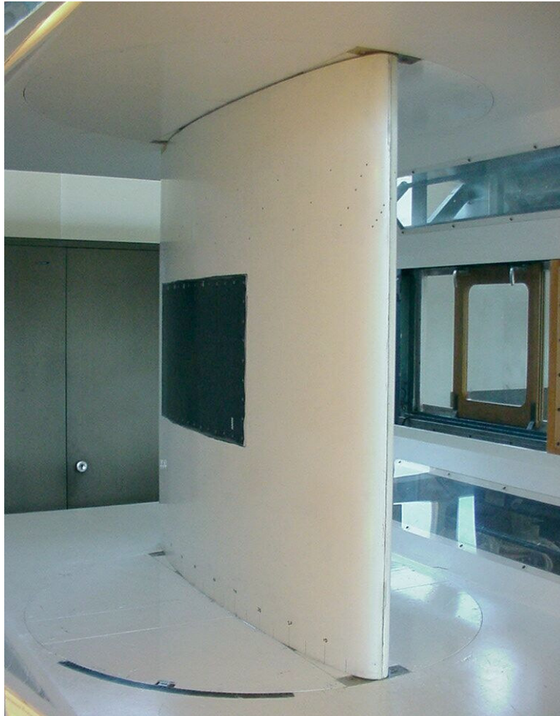
Fig. 3. Windtunnel model for boundary layer experiments in the interchangeable test section of the Low Speed Low Turbulence Windtunnel of TU Delft.
