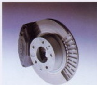
1. All-aluminium four-wheel double-wishbone suspension 2. Four-wheel ventilated disc brakes 3. Drilled aluminium brake pedal
